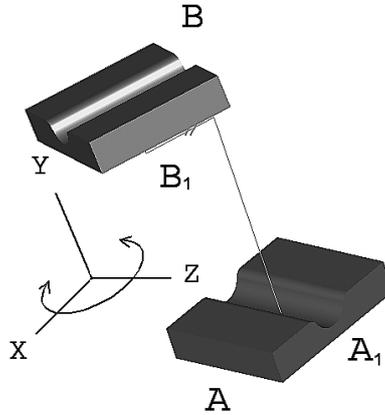
Figure 1. Relative degrees of freedom of two parts
