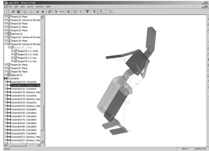
**Figure 6.** In LGS 3D, a model with 22 constraints is described by 9 equations only
