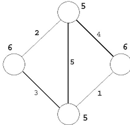
**Figure 4.** The maximal spanning-tree in a weighted graph
