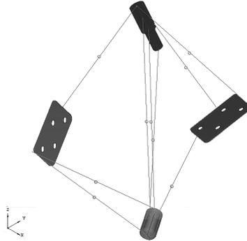
**Figure 2.** The initial model with 4 bodies and 9 constraints
