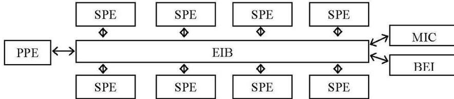
There is Element Interconnect Bus (EIB). The PPE and SPEs communicate coherently with each other and with main storage and I/O through EIB. The memory-coherent EIB has two external interfaces:
