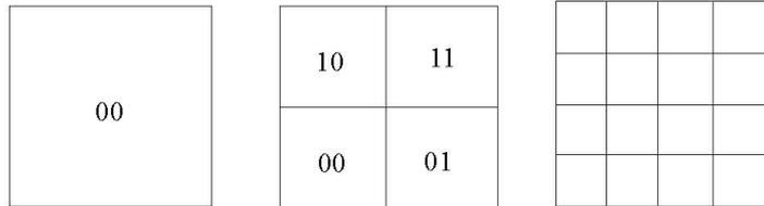
Every next partition is finer than the previous one. At the first step, there is no partition. The finest structure has rectangles consisting of one pixel. Some special structure will be associated with every partition.
