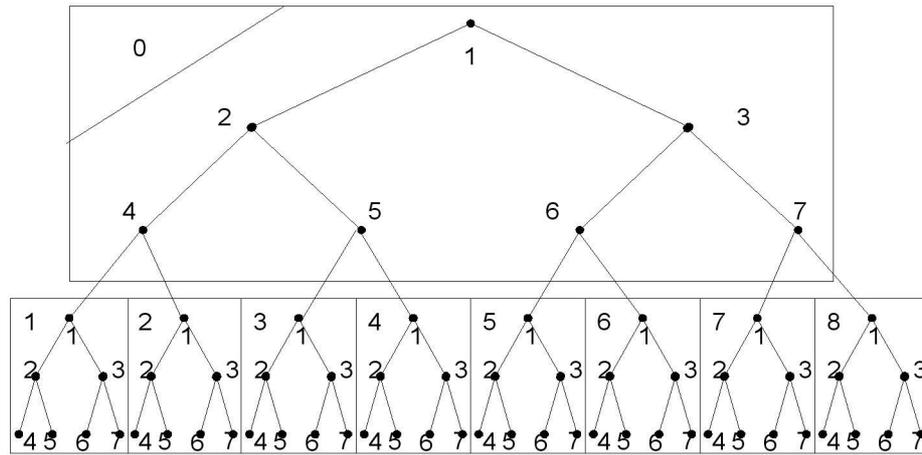
The correspondence between the vertexes of this tree and the cells of two-dimensional memory is rather simple.
