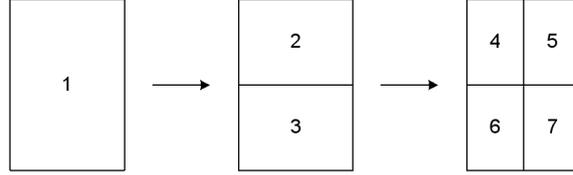
Every block breaks into 2 blocks at every next step. The partition types are alternated: at the beginning, it is vertical, then it is horizontal, etc.
