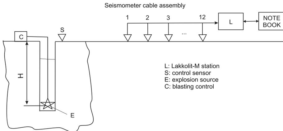
**Figure 1.** Scheme of model experiments
