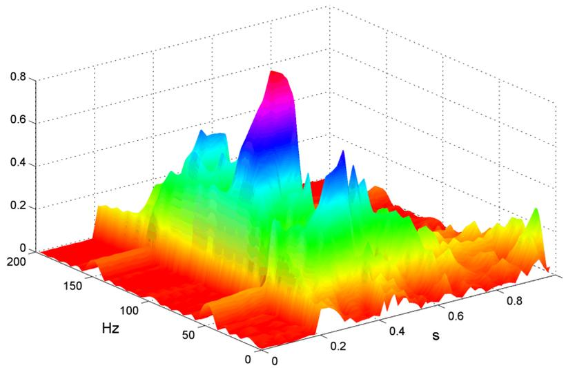
Figure 3. The spectral-time function of an explosion record at a depth of 100 m
