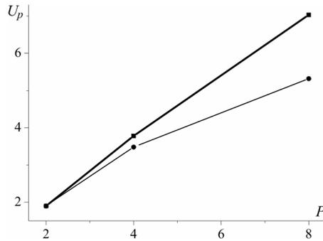
**Figure 3.** Acceleration of computation for  $5,000 \times 1,000$  grid spaces (circles) and  $10,000 \times 2,000$  (squares) for 2, 4, and 8 threads
