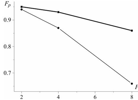
**Figure 4.** Efficiency of computation for  $5,000 \times 1,000$  grid spaces (circles) and  $10,000 \times 2,000$  (squares) for 2, 4, and 8 threads
