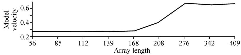
**Figure 14.** A change in the model wave velocity in ebonite-aluminium medium
