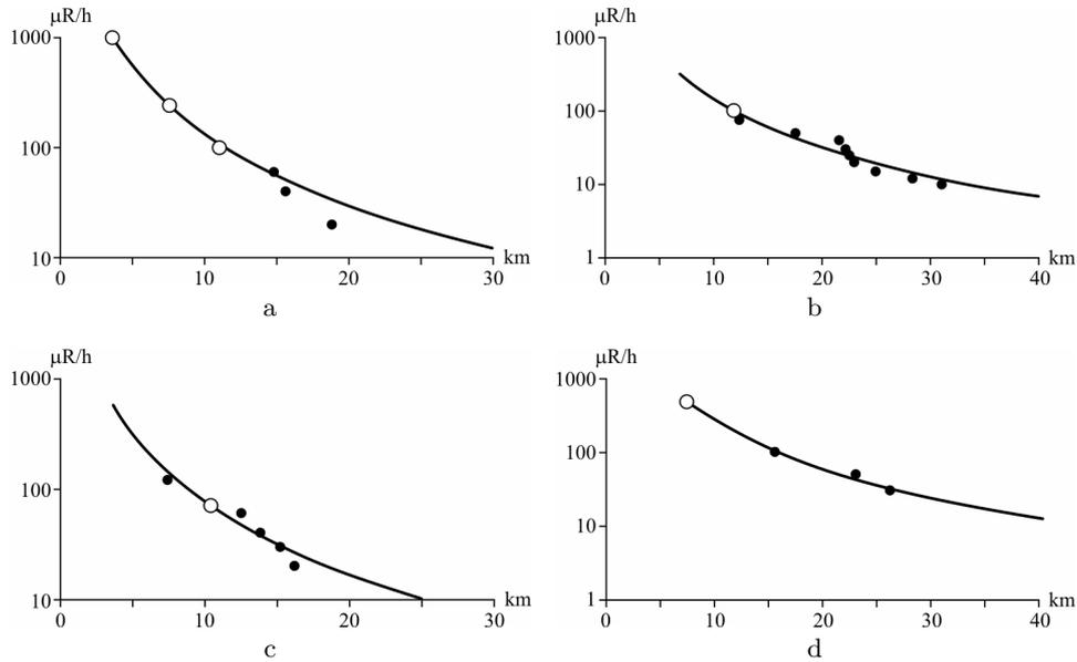
**Figure 2.** Levels of radioactive contamination of soil and snow cover resulted from the accident at the SCIC in 1993, that were numerically reconstructed from the observational data along the axis of the trace: a) May 13, b) April 12 (aero-gamma survey), c) June 13, d) April 12 (surface observations); — the result of numerical modeling; ●, ○ reference and control measurements points
