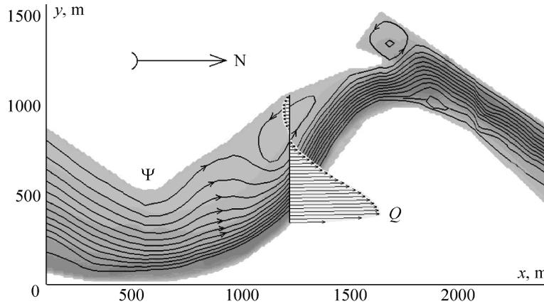
**Figure 1.** The current function isolines and the structure of a cross-section discharge (the central part) of the Ob river stretch near Barnaul city
