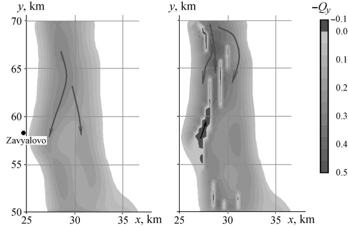
**Figure 2.** Spatial distribution of the discharge  $Q_y$  ( $\text{m}^2/\text{s}$ ) for the channel length of Novosibirsk storage reservoir near Zavyalovo village in no-wind conditions (left) and with north-east wind (right)
