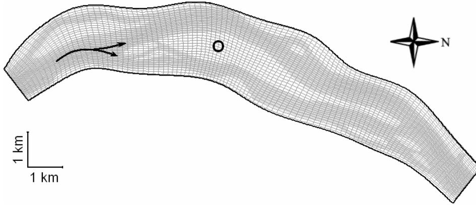
**Figure 1.** Grid structure of calculation area and channel contours of the Ob river (the grey tint)
