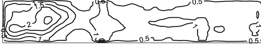
**Figure 6.** Electron density contours in the  $XY$  plane,  $z = L_Z/2$ , the moment of time  $t = 91.7$  (in terms of the plasma period). The density is given in terms of the initial values of density
