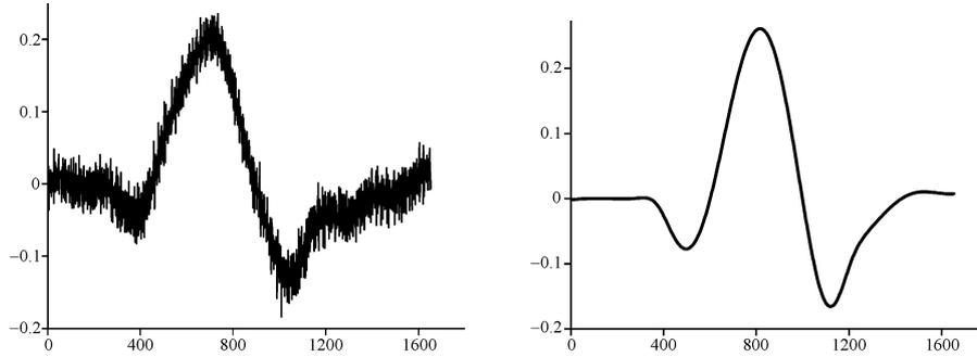
**Figure 3.** Typical signals with noise of 3% and the same signals after filtration
